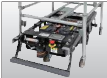
1 The AGV sneaks under the trolley.
